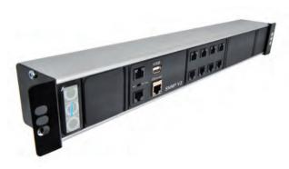
The OEC GATEWAY with SNMP V3 can connect all OEC PDU's in your datacenter / server room by RS485 or by the AP bus circuit / daisy chain system. The user-friendly embedded IP Web interface ensures full control over the system. OEC can also provide OEC Manager software for controlling multiple PDU installations, and by providing a MIB file OEC data can be read and used by third party management packages as well.
